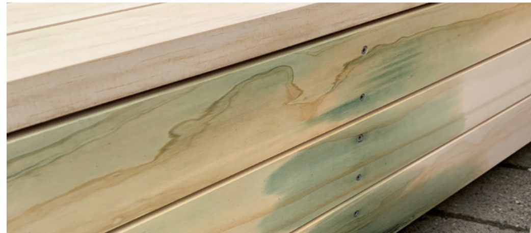
WICKING OF PRESSURE TREATED SOFTWOOD FRAMING CHEMICALS THROUGH ACCOYA
