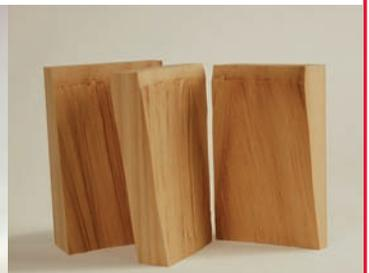
Sample: Accoya® wood scantling ... in delamination ... after delamination ... 100 % fibre-tear
