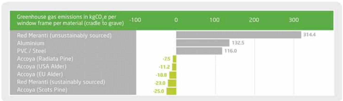
Figures 4 & 5: Greenhouse gas emissions for a window frame in various material alternatives
