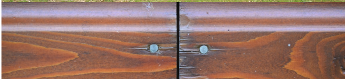
Siberian larch board showing end-grain fissures and discoloration at ends of boards due to water penetration after 5 years.
