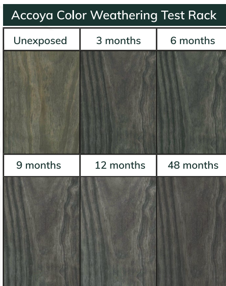
Accoya Color Field Exposure Trials tested in Corvallis, Oregon. *Please Note: Samples have not been cleaned. Annual cleaning or maintenance is highly recommended. See page 6 for more details.
