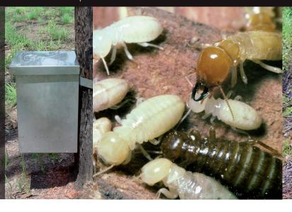
AWPC protocol for M. darwiniensis field testing in Humpty Doo, NT. Exposure chambers containing test wood are connected directly to active galleries of M. darwiniensis colonies. Tests run until termite activity in the chamber has ceased, and a minimum of 4-5 months.
