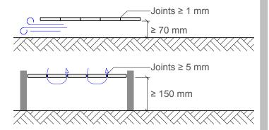
The centre-to-centre distance of a sub-frame depends highly on the board thickness the fixing system and the planned load. Wood decking for pedestrian use only and installed directly above a floor or the ground can be classified as a non-structural element, and a rule of thumb in determining the sub-frame distance 20 x the board thickness on centre.
