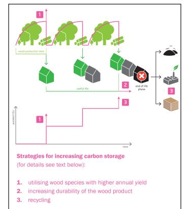
**Figure 4:** Avoided CO2 emissions in case of new sustainably managed plantations being established for manufacturing durable products (adapted after Technical University Munich, 2012)
