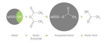
Figure 6: the chemical reaction occurring during acetylation
