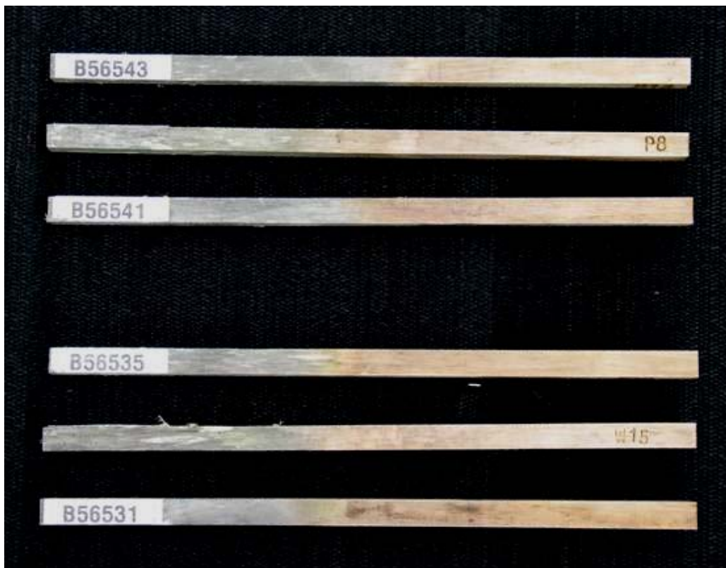
Figure 4 – The same stakes as in Figure 3 after six years exposure. While there was slightly more discoloration the stakes were still hard and appeared free from decay.
