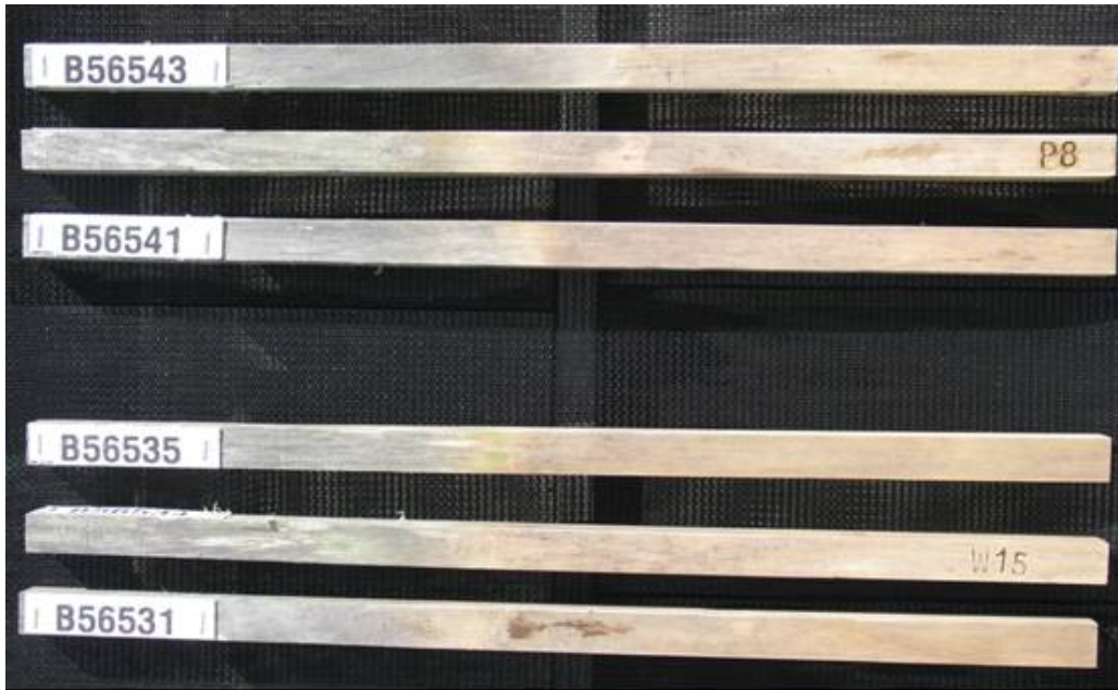
Figure 3 – Accoya pine stakes, from the LG031 treatment at the bottom and from the LG004 treatment at the top after five years exposure, showing weathering above ground and very little deterioration in the ground contact section.
