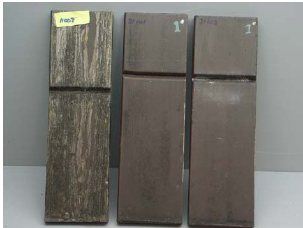
Untreated (left), acetylated and acetylated with residual acetic acid panels finished with a transparent teak coloured alkyd coating after 9½ years of outdoor exposure.
