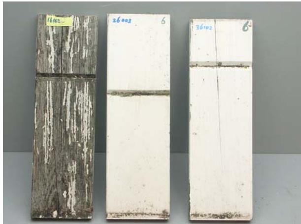
Untreated (left), acetylated and acetylated with residual acetic acid panels finished with an opaque white alkyd coating after 9½ years of outdoor exposure.
