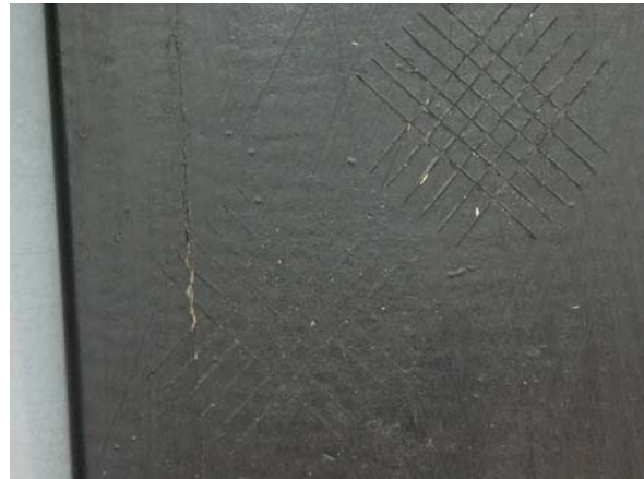
Adhesion test (ISO 2409) under wet (top) and dry conditions of acetylated (with residual acetic acid) Scots pine finished with an opaque dark alkyd coating after 9½ years outdoor exposure (sample 37003).
