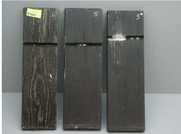
Untreated (left), acetylated and acetylated with residual acetic acid panels finished with an opaque black acrylic coating after 9½ years of outdoor exposure.
