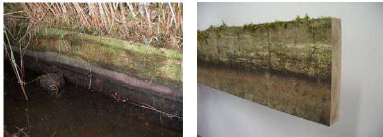
Figure 4. Acetylated poplar in test in a canal [left] and the sample after 13 years [right].
